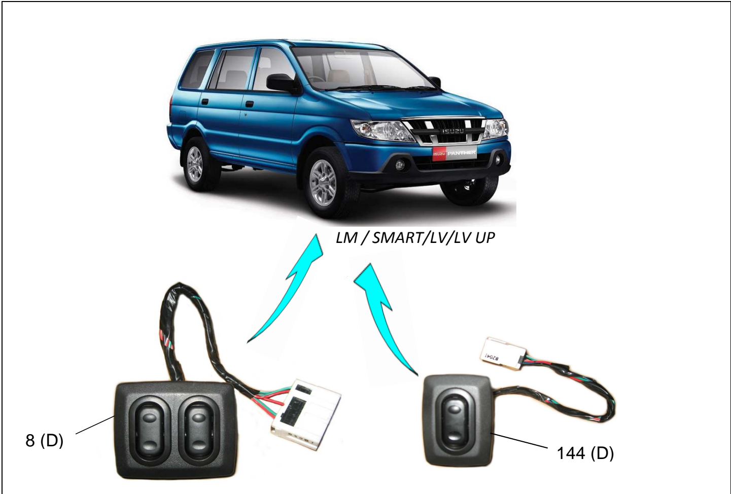
FIG.NO : 8-25 SWITCH AND RELAY; INSTRUMENT PANEL
